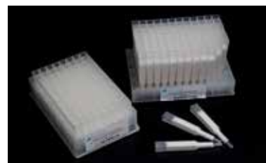
Cleanert® SLE plates Left: standard SLE plate; Right: Assemble SLE plate, up to 600 µL biosample can be load onto the plate.
